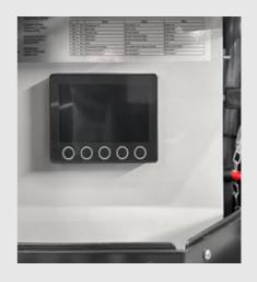
**OPERATING PANEL** WITH STATUS DISPLAY Keep an eye on everything: a protected display shows the most important Diesel engine data such as speed, consumption, temperature, and operating hours, visable at a glance.
