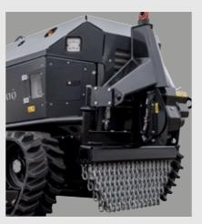
SAFETY A chain curtain provides additional protection against flying pieces of wood and stones.
