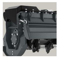
**PROTECTION FLAP** The optional flap on the front of the mulching head enables optimal mulching. It can provide extra protection by reducing uncontrolled ejection of mulched material.
