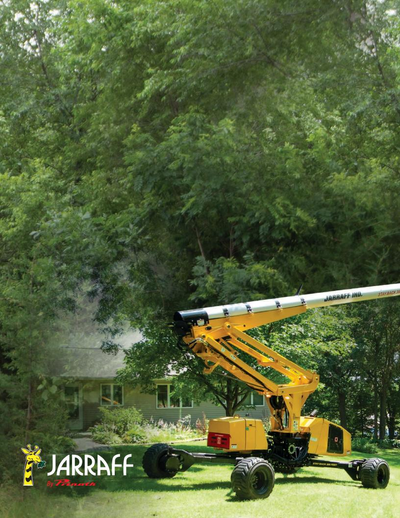
Self-leveling chassis, articulated steering, and wheels retractable from 10' to 42"; equals access to tight spaces and slope stability without outriggers.
