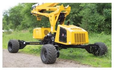
The Mini-Jarraff can easily navigate through difficult rural areas or urban locations. A **SELF-LEVELING CARRIER** allows the Mini-Jarraff to travel effectively on all types of terrain. Automatically adjusting legs narrow the machine's overall width to 48" and widen to 126" allowing the machine to work in the tightest of spaces, no outriggers required.
