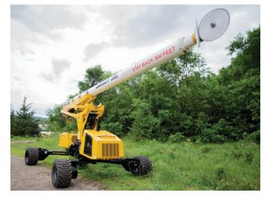
The unit offers **QUICK SET-UP** and a **DYNAMIC RANGE OF OPERATION** with extreme rotation and 15-degree manual leveling capability in all directions. The boom delivers a 55-foot vertical reach, providing **UNMATCHED CUTTING ABILITY**.
