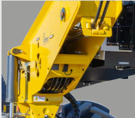
HYDRAULIC The internal hose reel optimally protects the important hydraulic hoses and valves from falling branches and dirt.
