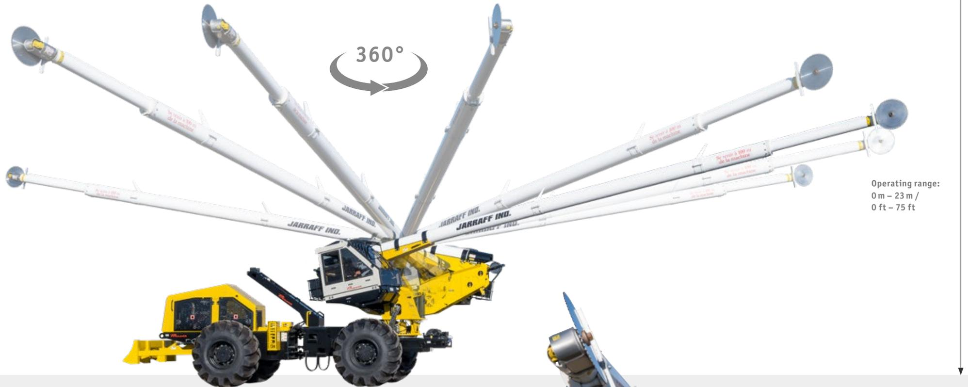
With its long boom and 180° tiltable saw blade at the end, the telescoping boom can effortlessly reach and cut branches up to 20 cm in diameter at heights of up to 23 m. The boom sits on a 360° swiveling slewing ring, which can also be swiveled sideways up to 40 degrees both directions during operation to optimally adapt to uneven terrain.
