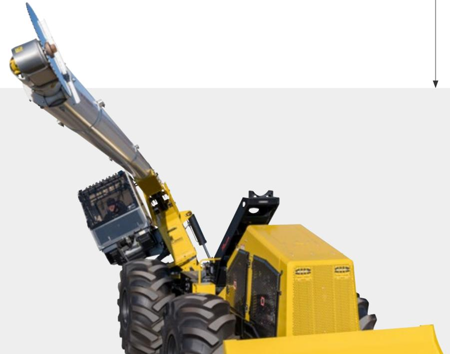
The unique design of the saw head allows the user to perform even difficult cuts quickly and in a controlled manner. The saw head can be rotated 180° – in combination with the lateral tilt of the cab, this enables precise work in all positions.
